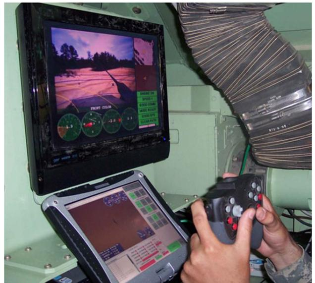
**Black Knight Unmanned Combat Vehicle** The National Robotics Engineering Center (NREC) developed sensing, teleoperation and autonomy packages for BAE Systems' Black Knight, a prototype unmanned ground combat vehicle (UGCV).
