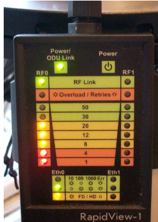
Link performance, signal display 20 we still have the link for level 4 @ +/- 45° miss pointed
