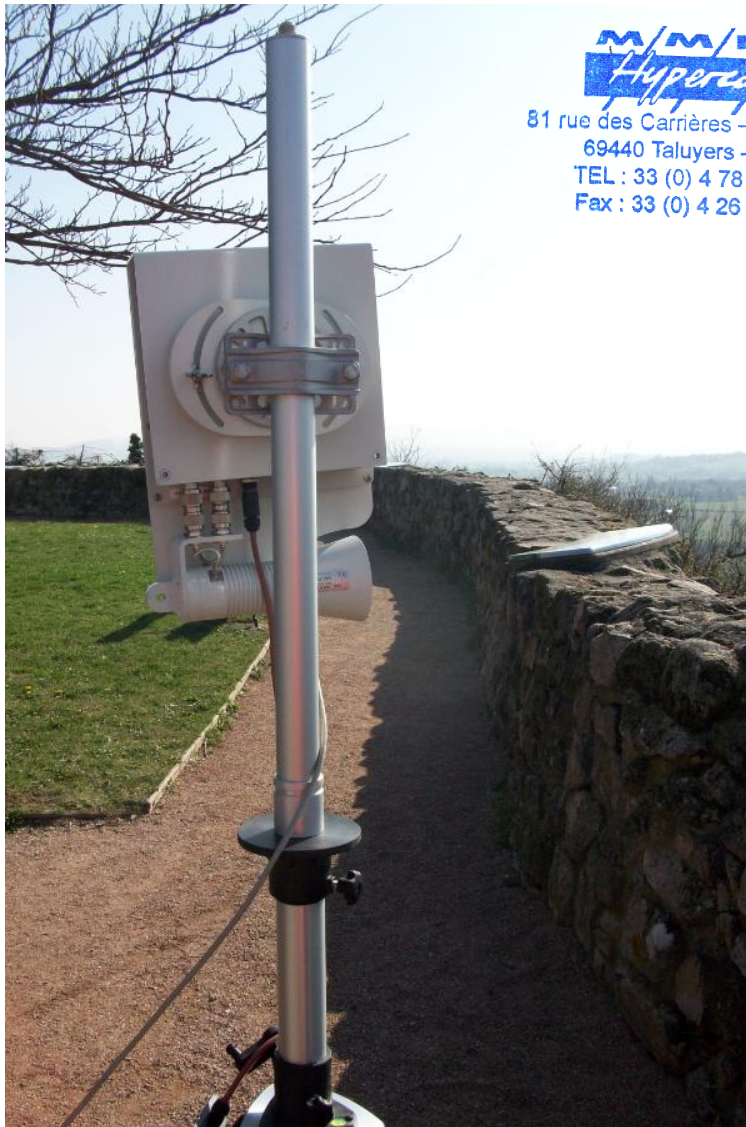
Link performance, signal display 20 we still have the link for level 4 @ +/- 45° miss pointed
