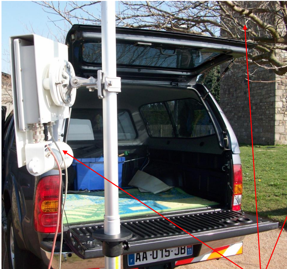
Link performance, signal display level 8 @ pointing to the stone building to receive in NO Line Of Sight beamed at reverse and only by reflexion
